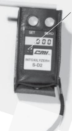
Unique indicator lights show the operator when the subject is providing a sufficient breath sample for analysis. The subject blows through the mouthpiece until both the "A" and "B" lights are illuminated. The operator then presses the "READ" button until the alcohol reading is displayed.
