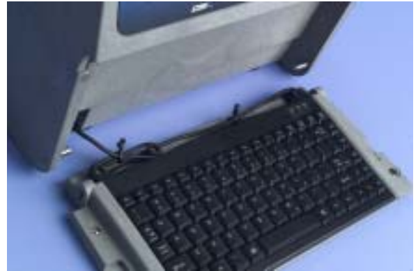
The integral keyboard detaches for easy use and test subject data entry.
